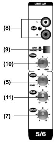
For example, with the Balance control turned fully clockwise, only the right portion of the channel's stereo signal will be routed to the Master Mix.
